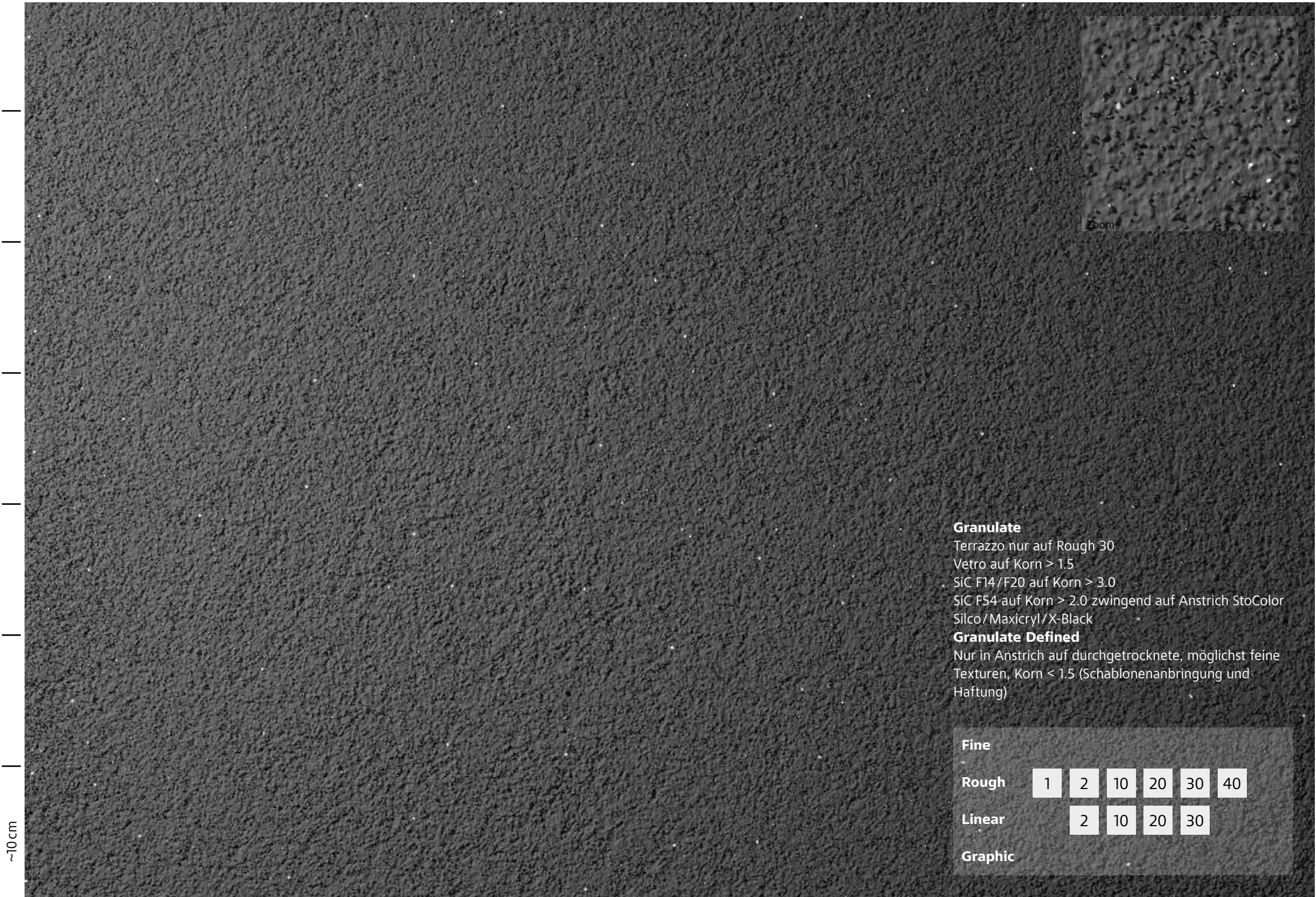
Texture: Rough 1, Stolit K 3.0 (37104) + Effect: Granulate 30, StoColor Silco (37104)/Sto-Siliciumcarbid F20
